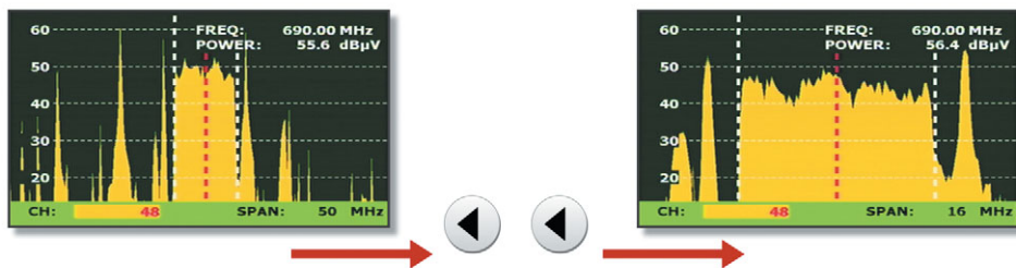
By pressing LEFT key twice, the instrument sets the SPAN from 50 to 16 MHz
